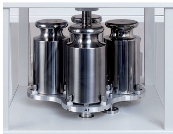
Weight positioning of sliding nature prevents errors of eccentricity.
