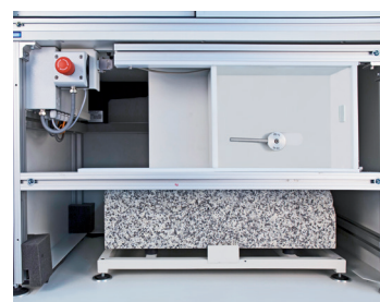
Sturdy design of the table, featuring heavy granite stone and robust rubber shock absorbers, reduces effect of vibrations to the absolute minimum.
