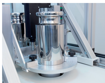
Dedicated weighing pan design facilitates extremely precise weights comparison, no matter how light the weights are.
