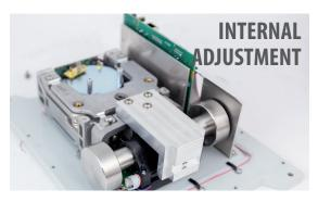
An internal automatic adjustment system quarantees measurement repeatability and precision even under changing ambient conditions.
