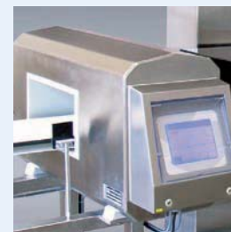
Tunnel metal detector
