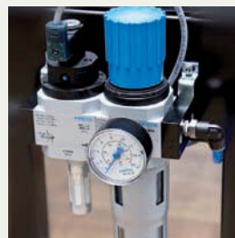
Compressed Air Service Units
