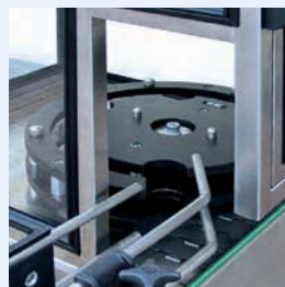
Rotational feeder of cylindrical products
