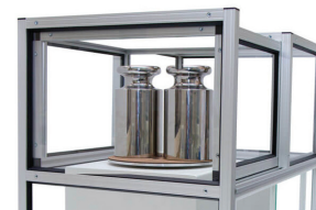
Mass standards in mass comparator chamber during comparison
