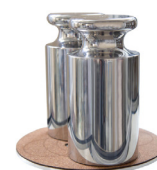
Mass standards on self-centring weighing pan
