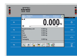
PUE 7.1 indicator with 5.7" colour graphic display
