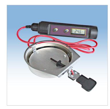
The main parameter determining the result of humidity content in a tested sample is the drying temperature. Placing the control thermometer directly above the drying pan enables reading the temperature close to the one of the tested sample. Thus, the adjustment is carried out in actual thermal conditions occurring on a typical analysis. A moisture analyzer adjusted using the control thermometer GT105k-12/Z series operates precisely and with the highest accuracy.
