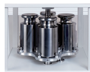
Positioners facilitating precise loading of weights
