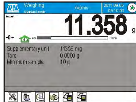
Weight value higher than the MSW value specified for a particular tare range.
