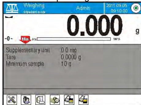
Weight value lower than the MSW value specified for a particular tare range.
